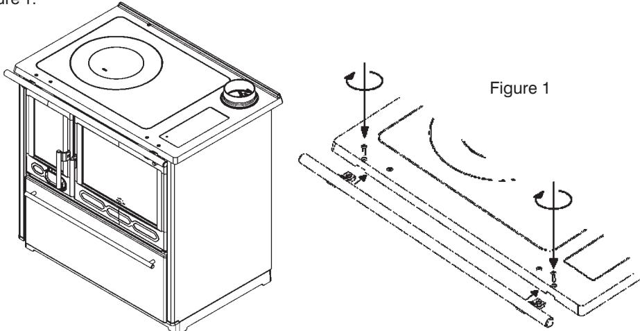
Install the flue collar in its position making sure that the connection between the cookstove and chimney is firm and tight. The cooker is connected to the chimney with a standard flue pipe dia. 120 mm. The flue pipes should have adequate rise at all places. Do not connect the cooker to a chimney to which another appliance has already been connected. Make sure that the chimney is free from any cracks and damages.
