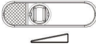
To operate the fireplace at the minimum output, set the primary air supply control to fully closed position. If you have a fluepipe damper installed, close the damper as well.
