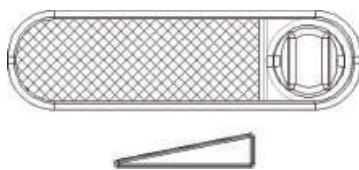
When the fire has blazed up and sufficient ember bed has been created, set the air supply control back to the position ensuring the air supply that is sufficient for the fireplace to develop as much heat as required.
